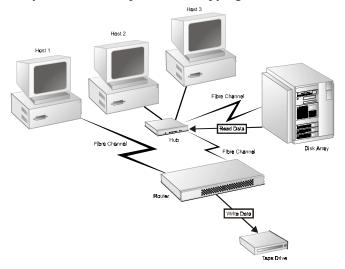
Figure 2-10. Extended copy configuration example
